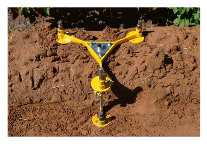
Two Tripod Feet are secured near the top of the hill, while the Extension Foot is secured at the bottom of the furrow.
