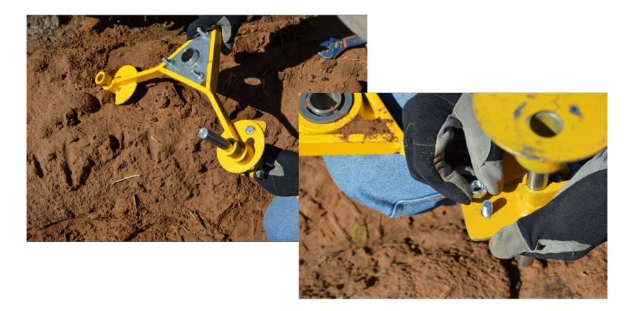
Align the holes of the Tripod Foot and the Extension Foot, insert the bolt through the holes and tighten with the nut.
