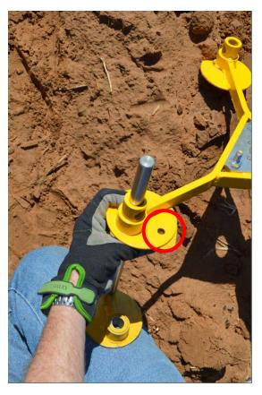
Insert the Extension Foot into the Tripod Foot (white circled). Use the Tripod Foot with the pre-drilled hole (red circled).
