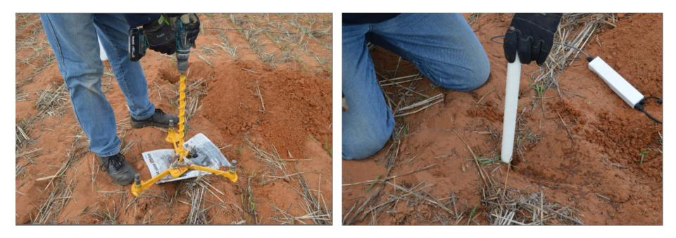
Use the 30cm Installation Auger and Tripod. As before, check the hole depth, make a 3cm deep channel for the probe cable next to the probe, lubricate the probe with a little water and insert it. The cable may also be installed in a 20cm deep trench, but is more conveniently left on the surface so that the probe may be removed to one side temporarily at harvest and planting times.
