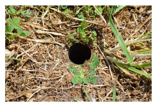
It is not possible to achieve the quality and integrity of the drilled hole (as shown in the picture above) without using the Sentek Stabilisation Tripod for the tapered auger.
