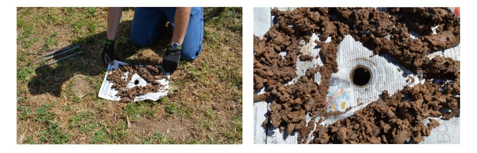
Remove the tripod and inspect the quality of the hole. It should be smooth-sided and free of air pockets. Carefully remove the augered soil from the site using the newspaper.
