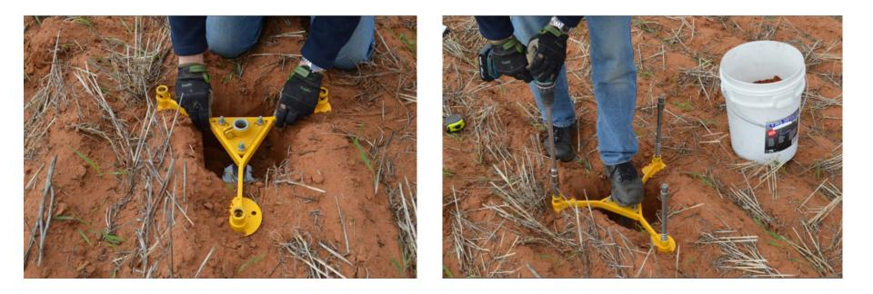
Position the Extension Tube in the centre of the excavated hole and install the Screw Pins.
