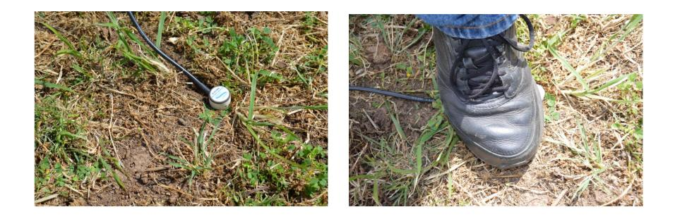
If the probe protrudes above the soil surface and you cannot push it any further by hand, gently step on it and use your body weight to push it into final position. Do not use unreasonable force.
