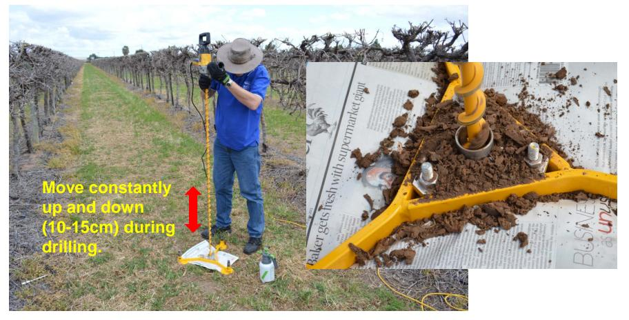
Insert the auger into the centre of the tripod keeping it as straight as possible. Start the drill and move the auger constantly and gently 10 - 15 cm up and down during the drilling process. This enables movement of the soil from the auger flight upwards and out of the drilled hole.
