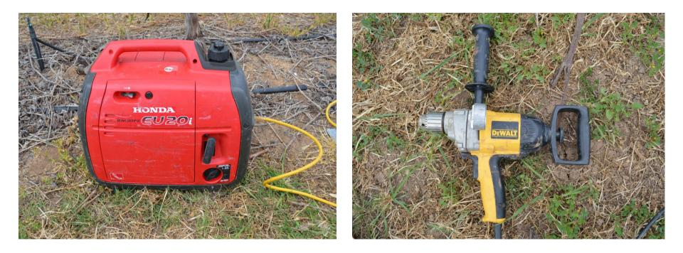
A Honda EU20 i 1.6 KVA Generator and a 740 Watt DEWALT Drill have been intensively tested to drill holes in some very heavy textured soils. These tools have not failed in the course of many installations and are highly recommended.
