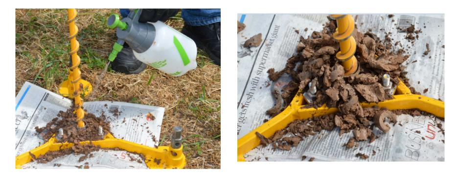
When the going gets tough in heavy soil, spray some water onto the auger and into the hole.
