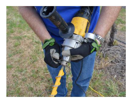
Insert the Tapered Auger into the drill and tighten the drill chuck.
