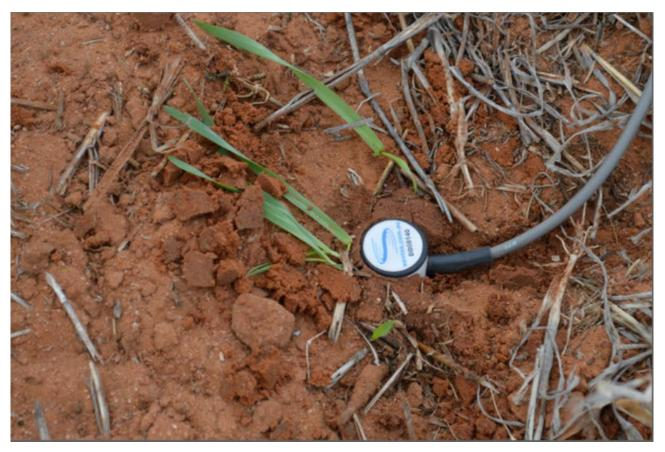
The almost-completely installed 30cm probe. The probe cable can be fitted with protective electrical cable conduit and buried adjacent to the probe. The cable can be left on the surface for convenient removal at times of farm machinery traffic.
