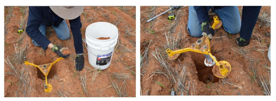
Before removing the tripod, remove any soil that may have landed in the hole around the Extension Tube. This will protect the augered probe hole during removal of the Tripod.
