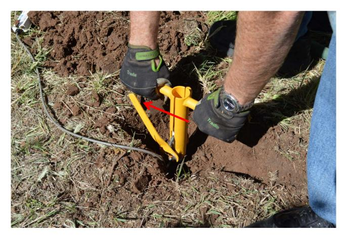
Move the lever of the tool from left to right as far as possible, being careful not to damage the probe cable. Grab the tool handle and pull with a <u>gentle</u> twisting motion to remove the probe.
