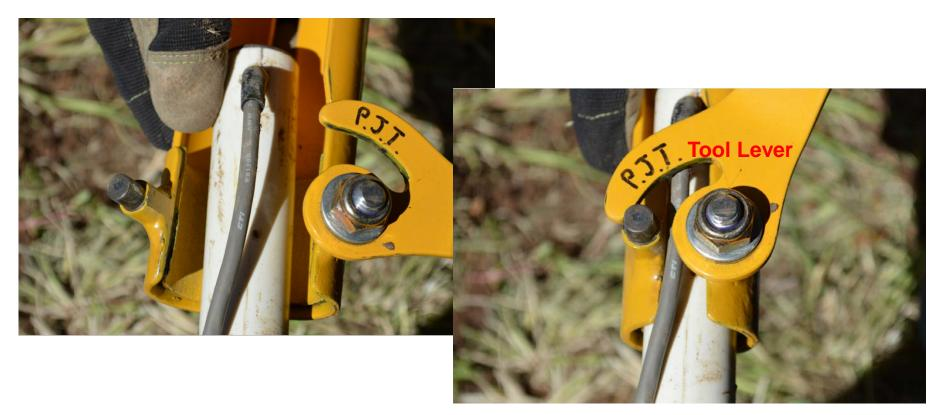
In close-up: Locate the probe cable in the square opening of the extraction tool and hold it against the probe body below the tool lever as shown. Line the probe cable up with the split in the Extraction Tool. This is done so that in the event of tool slippage, the cable will not be sheared off.
