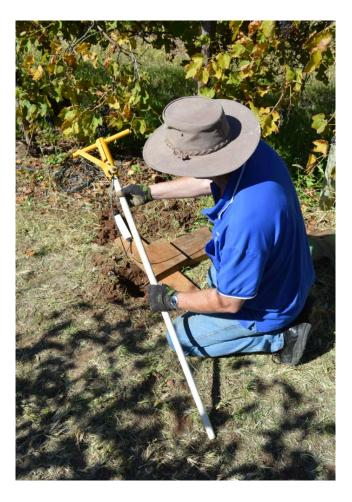
Gently remove the Drill & Drop Probe when it becomes free of the soil.
