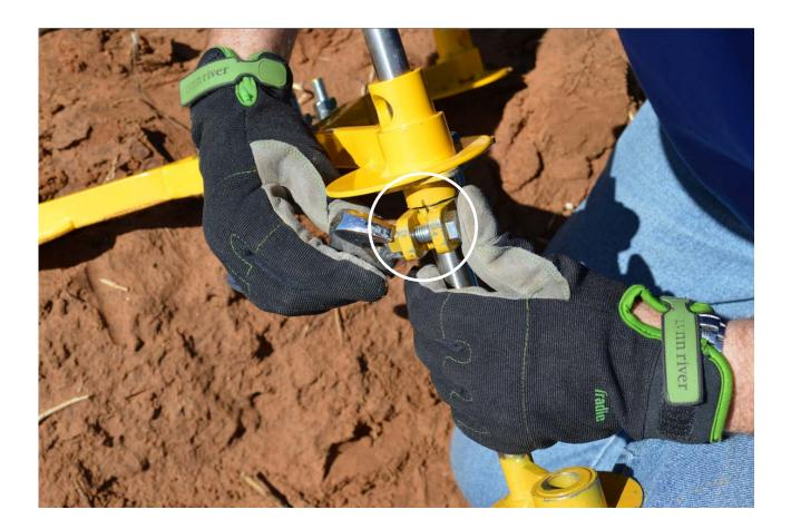
Re-tighten the nut and bolt (circled).
