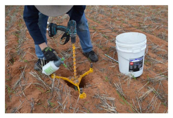
Use a water spray bottle to lubricate and pick up the augered soil. Auger in short stages (30–50cm at a time), clearing the auger flights regularly. The excavated soil should be moist to maintain the integrity of the hole. Dry soil will collapse inward and lead to air gaps and failure of probe insertion.
