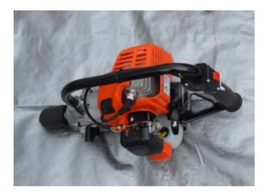
Alternatively, a motorised power head may be used to drive the tapered auger. The one shown is an ECHO EDR-2400 2-stroke engine drill by Yamabiko Corporation.
