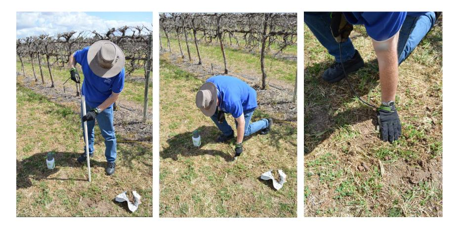
Insert the probe carefully into the hole pushing it all the way down until the top of the probe is level with the soil surface. The first sensor will now be located at 5cm depth.
