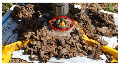
Now reintroduce the auger carefully with the drill switched off. Push the auger until the top end of the flight is level with the hole of the tripod. If the auger will not go down to this level, give the auger a quick spin to take up the soil at the bottom of the hole, then stop the drill, remove it from the hole carefully and clean it once again.
