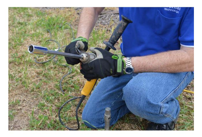
Place the Socket Tool into the drill and tighten the drill chuck with the chuck key.
