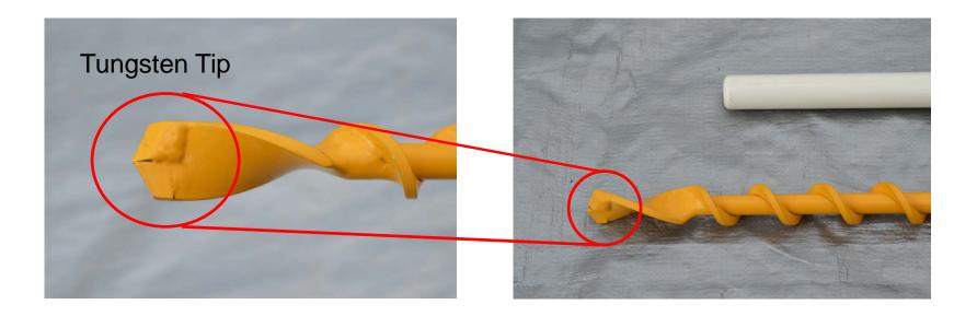
The tungsten-tipped auger is a little longer than the probe. The tapered soil opening created by the auger is therefore deeper compared to the length of the probe body. The resulting soil cavity below the bottom of the probe is designed to accept any soil accumulating at the bottom of the cavity during the installation process. Otherwise soil accumulation could obstruct the insertion of the probe body to its full length.
