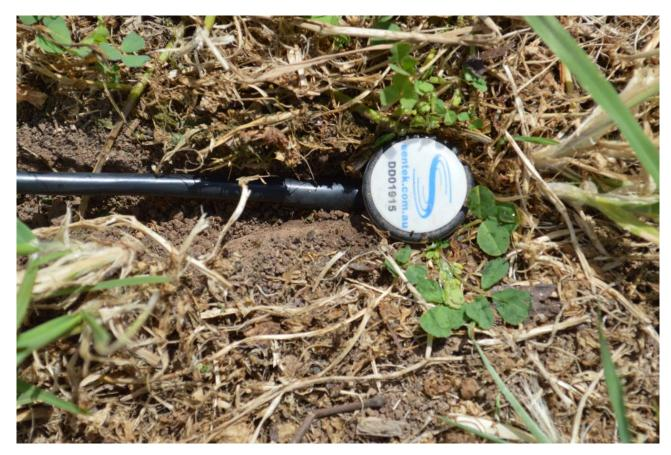
The (almost) completed installation of the probe should look like this. The probe should be in firm contact with the soil and you should not be able to push it in any further by hand. Last thing: The channel for the cable should be filled with soil.
