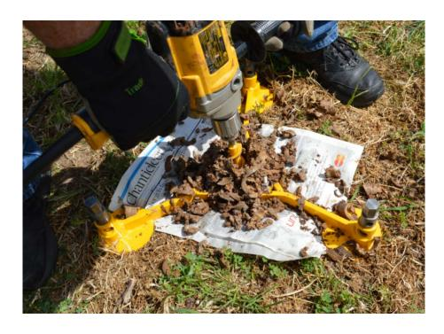
Auger until the end of the auger flight is level with the top of the bush of the tripod and stop the drill. Then carefully remove the auger from the hole.
