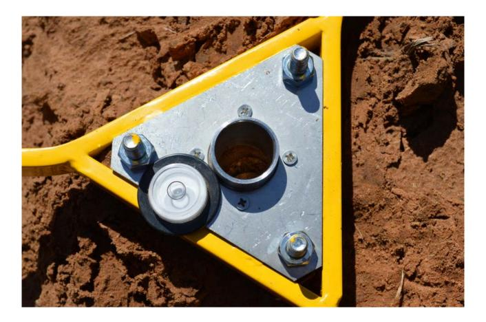
Use a levelling bubble to position the tripod correctly.
