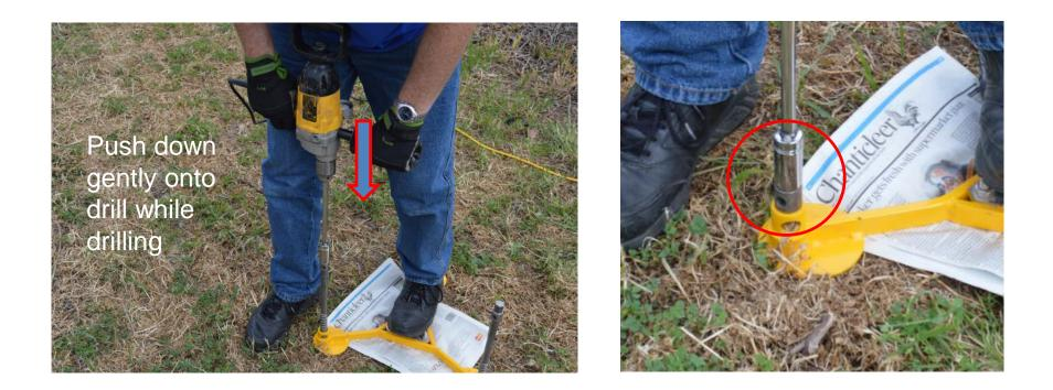
Place one foot onto the centre of the tripod, position the Socket Tool onto the Screw Pin and keep drilling until the head end of the pin comes to rest on top of the tripod. Repeat with the remaining 2 Screw Pins and then check the tripod stability manually.
