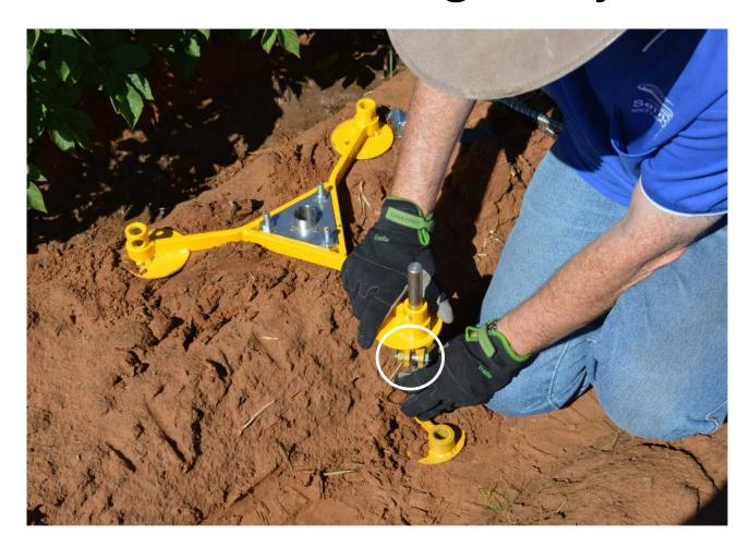
Loosen the nut and bolt of the height clamp (circled) and slide the leg to the desired height.
