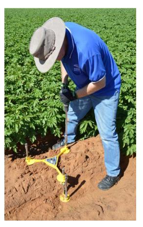
Insert the Tripod Screw Pins into the holes in the Tripod Feet and Extension Foot. Use an electric drill to secure the two Tripod Feet on the hill ridge and the Extension Foot in the furrow.
