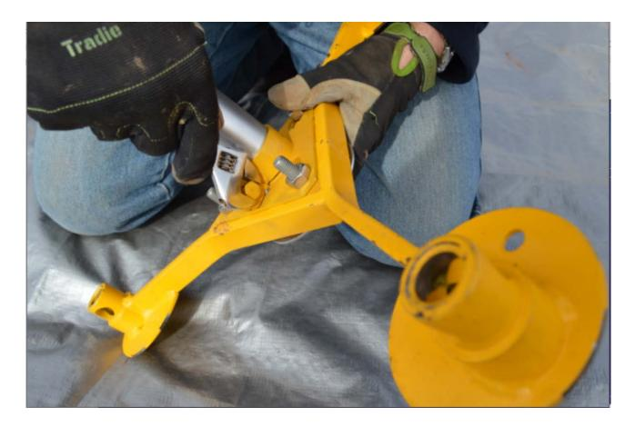
Loosen the Extension Tube nut to release the Extension Tube.
