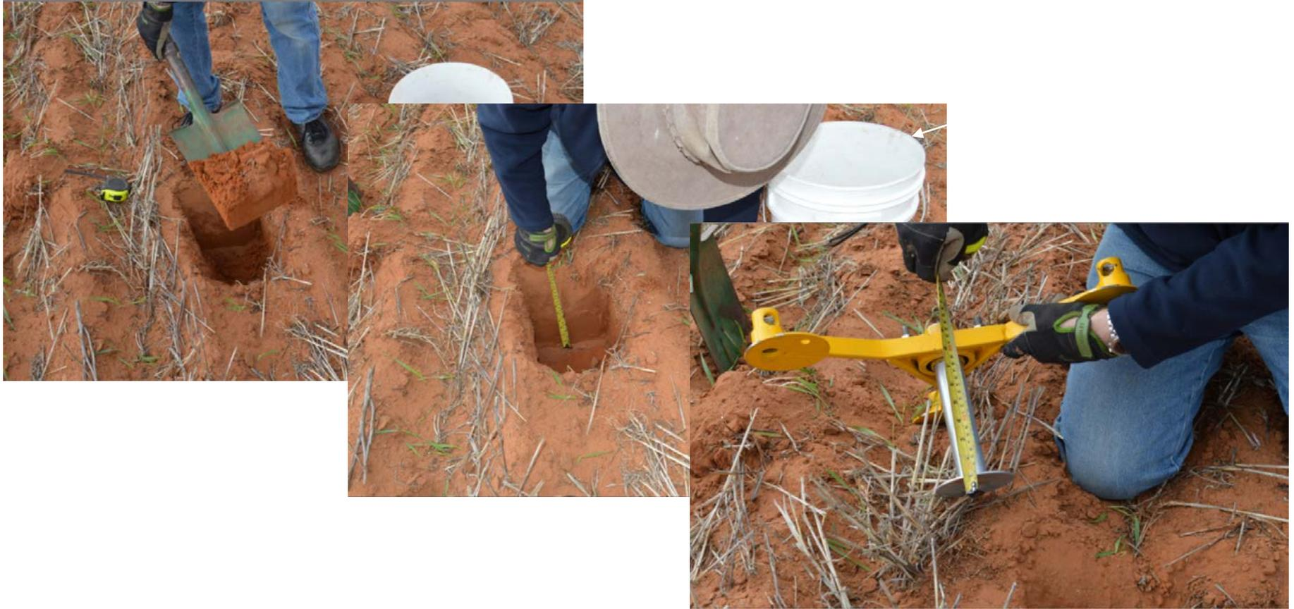
Excavate the soil to the correct depth. Ensure that the bottom of the hole is level.
