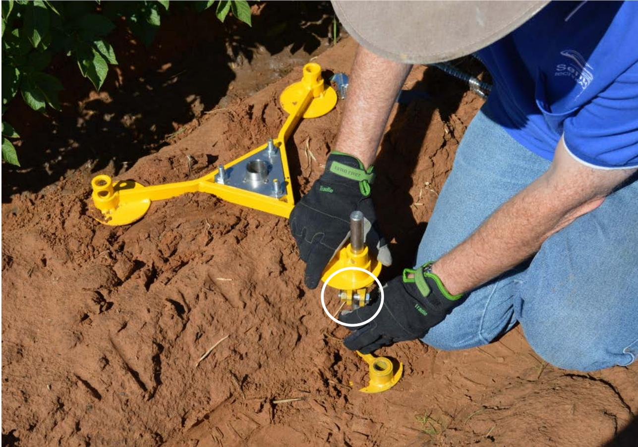
Loosen the nut and bolt of the height clamp (circled) and slide the leg to the desired height.
