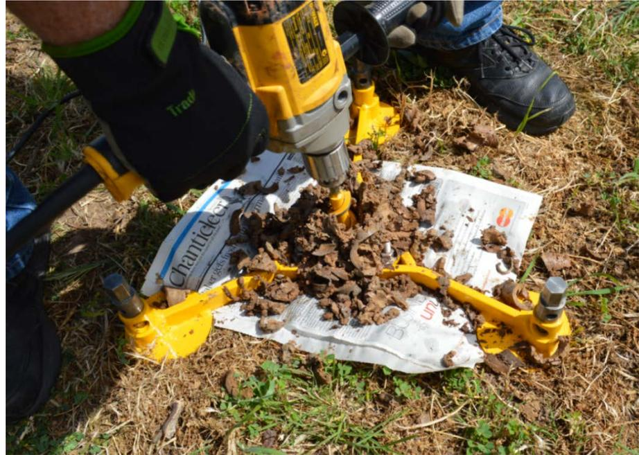
Auger until the end of the auger flight is level with the top of the bush of the tripod and stop the drill. Then carefully remove the auger from the hole.
