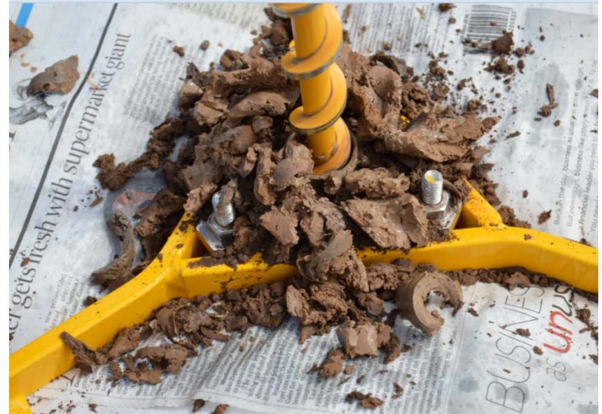
When the going gets tough in heavy soil, spray some water onto the auger and into the hole.
