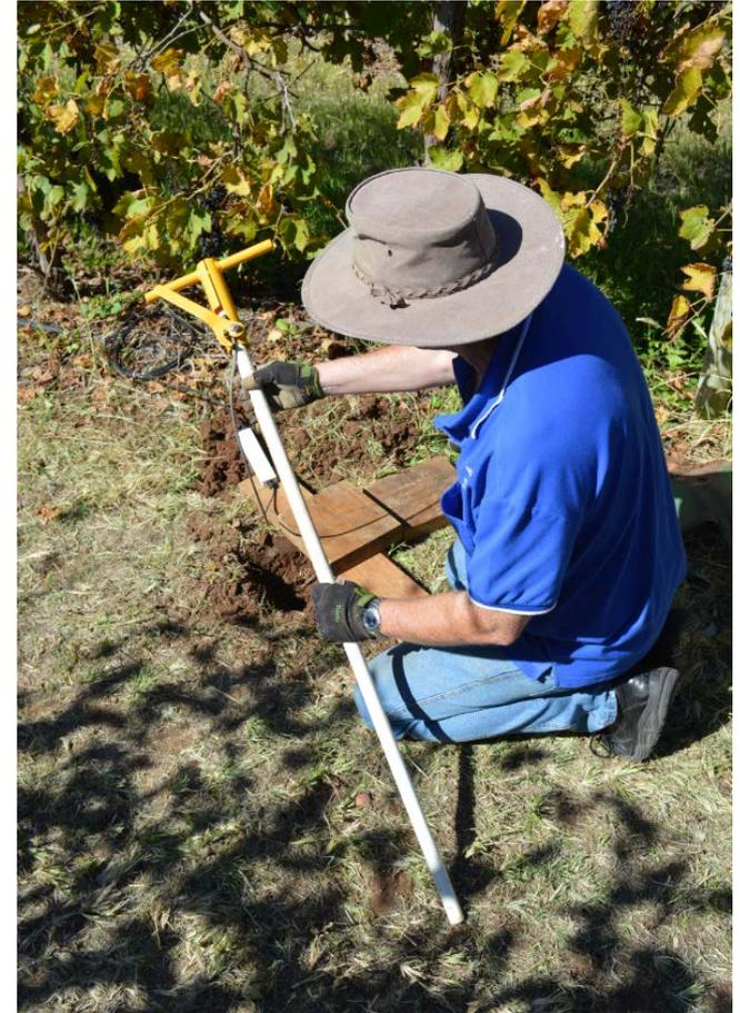
Gently remove the Drill & Drop Probe when it becomes free of the soil.
