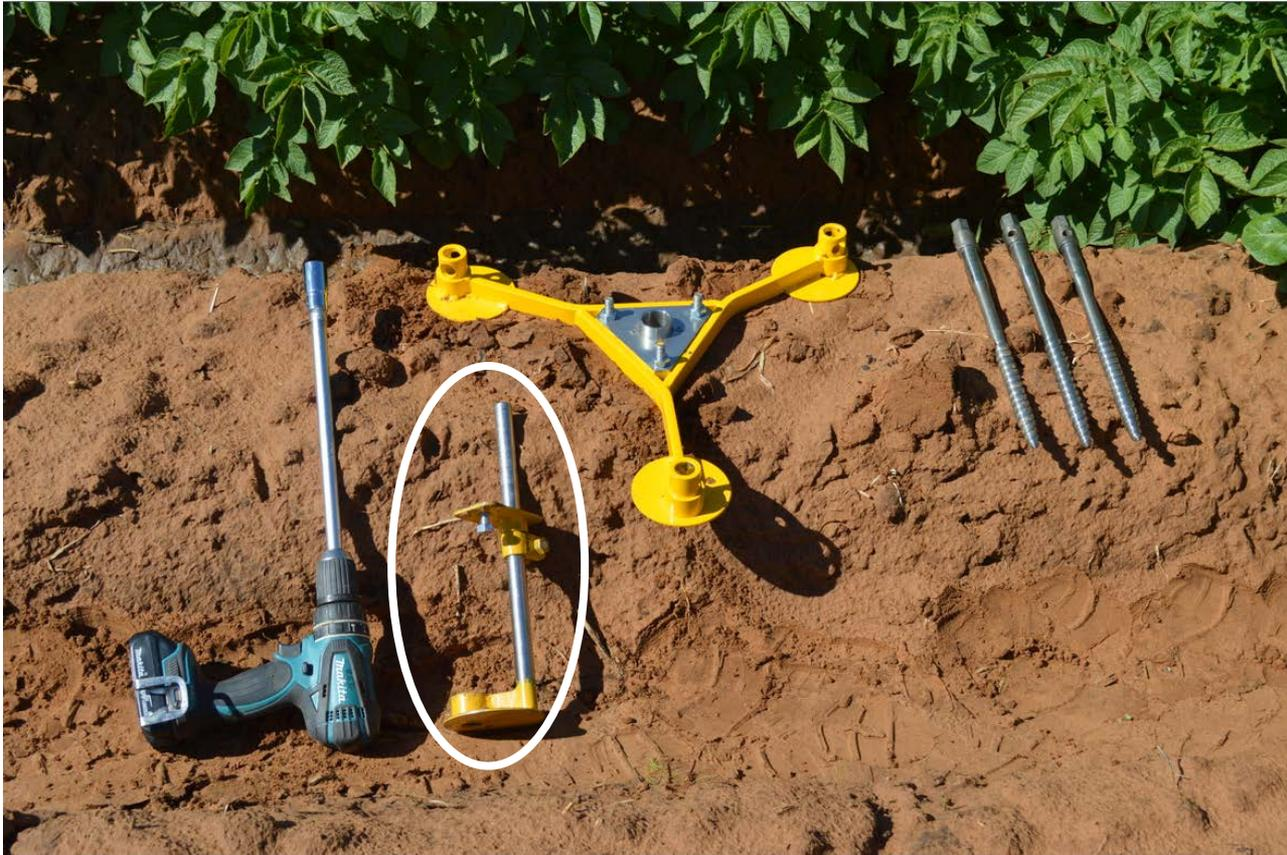
When installing the Drill & Drop probe in crops grown on hills an Extension Foot (circled) is used to stabilise the Tripod on the hill ridge.
