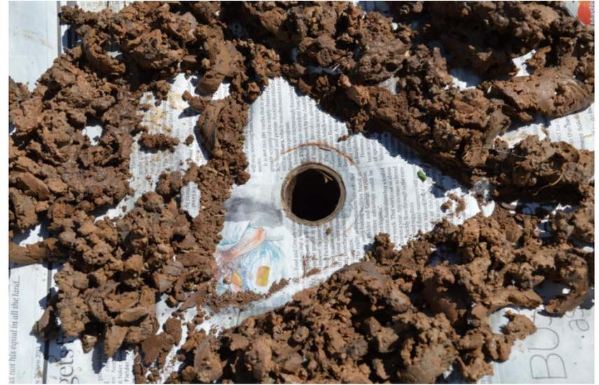
Remove the tripod and inspect the quality of the hole. It should be smooth-sided and free of air pockets. Carefully remove the augered soil from the site using the newspaper.
