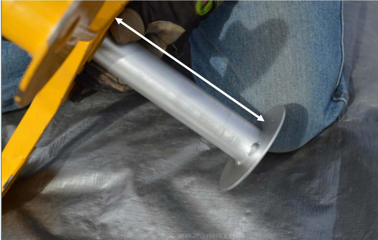
Adjust the Extension Tube to the desired depth of the probe below the surface (white arrow) and tighten the Extension Tube nut.
