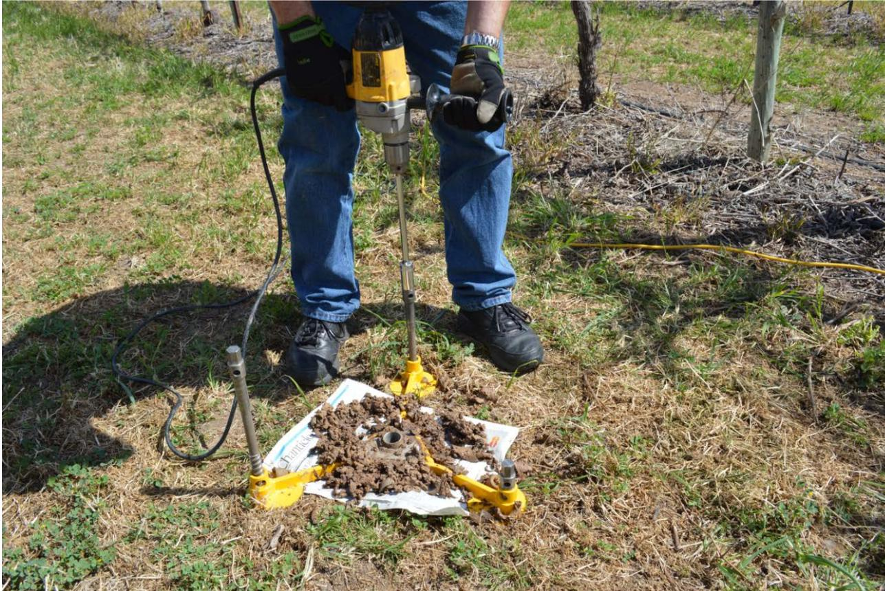
Use the drill in reverse mode to unscrew the pins.
