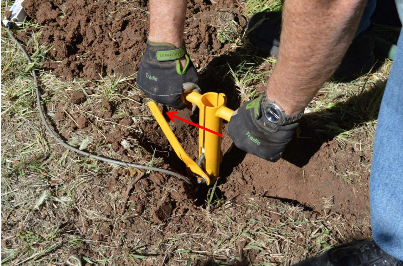
Move the lever of the tool from left to right as far as possible, being careful not to damage the probe cable. Grab the tool handle and pull with a gentle twisting motion to remove the probe.
