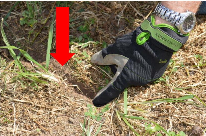
Use a small trowel to dig a trench to accept the probe cable. During excavation, place your finger over the hole to prevent any soil falling in.
