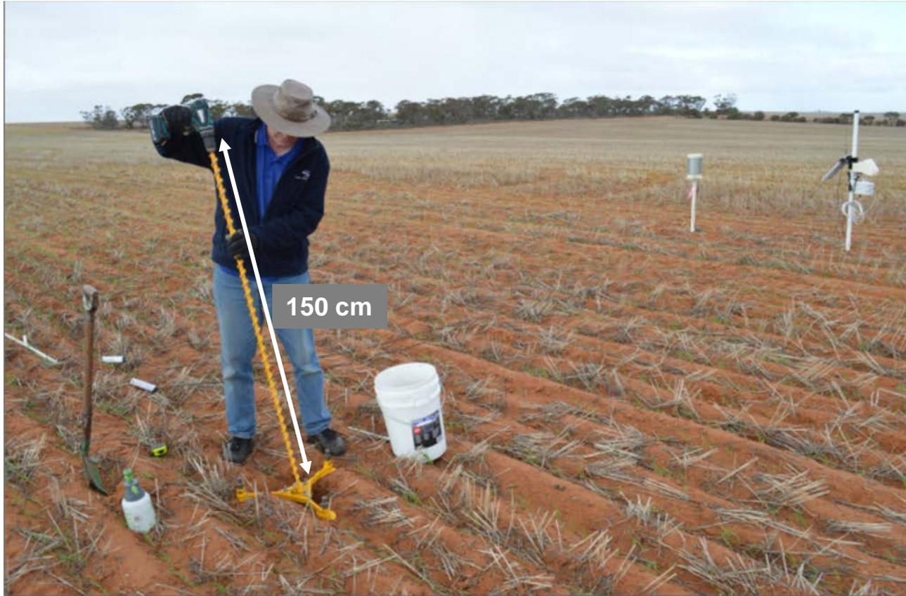
Use the extended 150cm subsurface auger. Measure and mark the auger at the required depth. Allow for the tripod centre height of 4cm.
