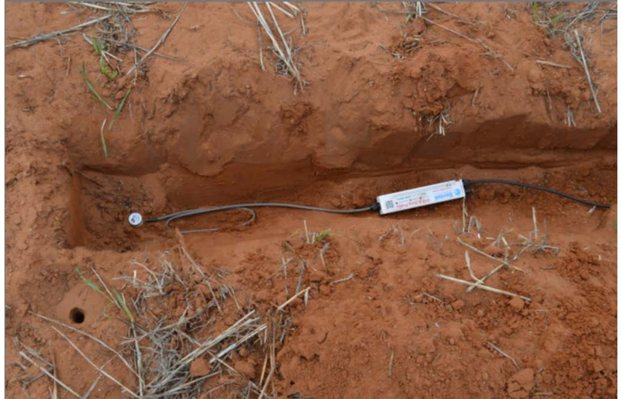
The entire cable is placed in a 20cm deep trench to protect it from cultivation tynes.
