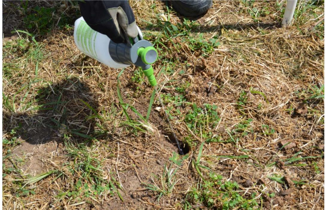
Use the spray bottle to wet the probe and the upper walls of the hole. This is particularly useful as lubrication in clay soils.
