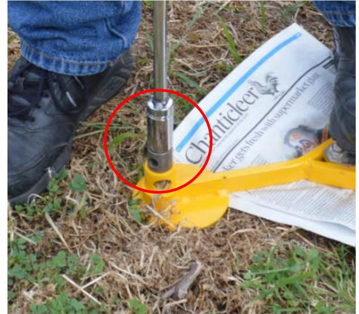
Place one foot onto the centre of the tripod, position the Socket Tool onto the Screw Pin and keep drilling until the head end of the pin comes to rest on top of the tripod. Repeat with the remaining 2 Screw Pins and then check the tripod stability manually.
