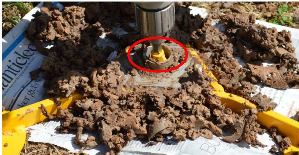
Now reintroduce the auger carefully with the drill switched off. Push the auger until the top end of the flight is level with the hole of the tripod. If the auger will not go down to this level, give the auger a quick spin to take up the soil at the bottom of the hole, then stop the drill, remove it from the hole carefully and clean it once again.
