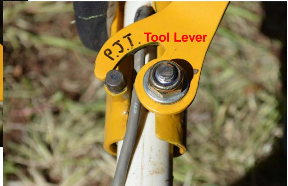
In close-up: Locate the probe cable in the square opening of the extraction tool and hold it against the probe body below the tool lever as shown. Line the probe cable up with the split in the Extraction Tool. This is done so that in the event of tool slippage, the cable will not be sheared off.
