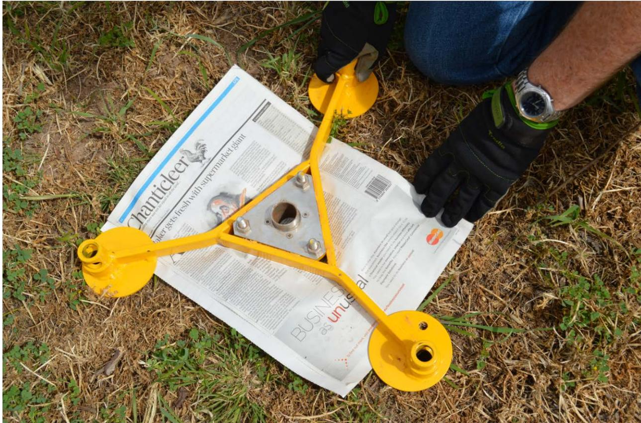
Place 2 sheets of newspaper beneath the Stabilisation Tripod. This allows easy removal of the augered soil later.
