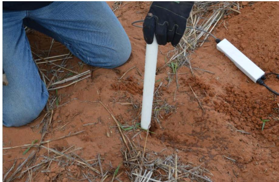
Use the 30cm Installation Auger and Tripod. As before, check the hole depth, make a 3cm deep channel for the probe cable next to the probe, lubricate the probe with a little water and insert it. The cable may also be installed in a 20cm deep trench, but is more conveniently left on the surface so that the probe may be removed to one side temporarily at harvest and planting times.
