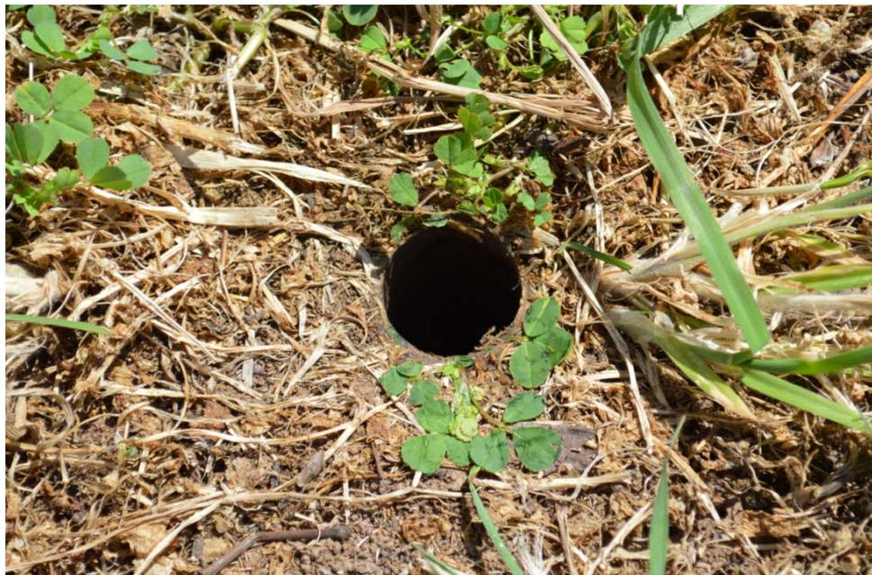
It is not possible to achieve the quality and integrity of the drilled hole (as shown in the picture above) without using the Sentek Stabilisation Tripod for the tapered auger.
