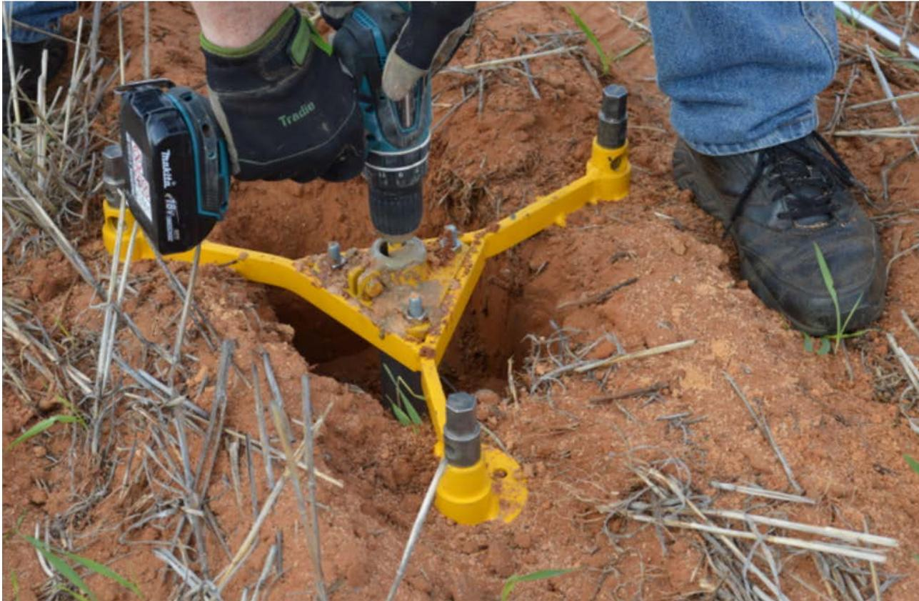
Drill to your auger mark, then carefully take the auger out, remove any soil from it and re-insert it back into the hole without rotating it. If you can insert it all the way then the hole is deep enough to receive the probe. If not then carefully auger more soil out and retest until sufficient depth is reached.
