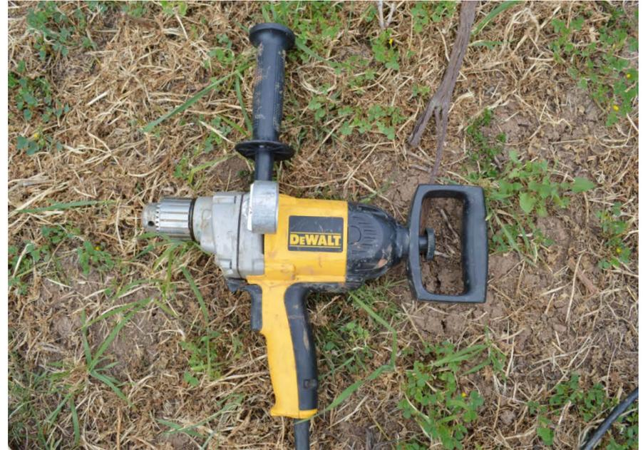
A Honda EU20 i 1.6 KVA Generator and a 740 Watt DEWALT Drill have been intensively tested to drill holes in some very heavy textured soils. These tools have not failed in the course of many installations and are highly recommended.
