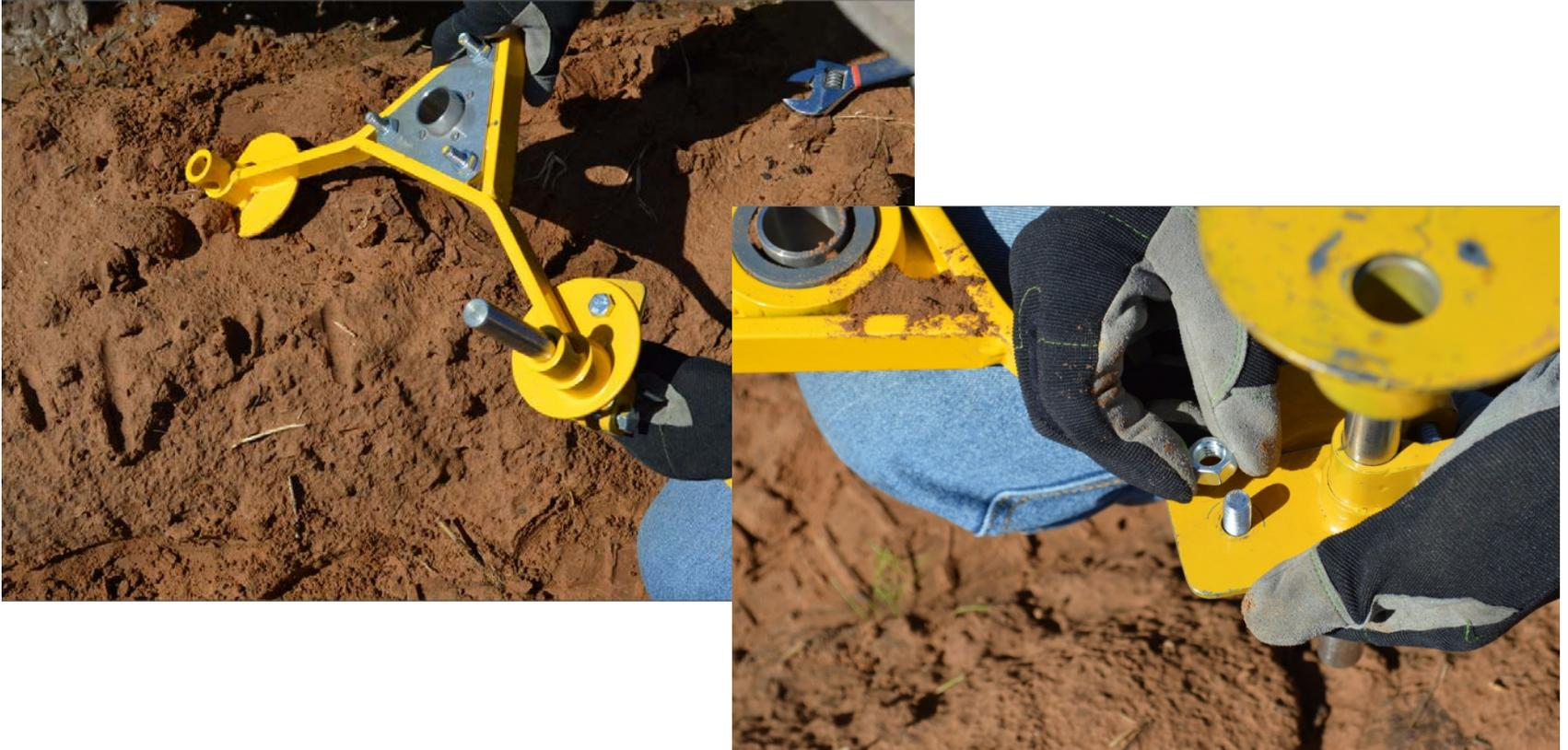
Align the holes of the Tripod Foot and the Extension Foot, insert the bolt through the holes and tighten with the nut.
