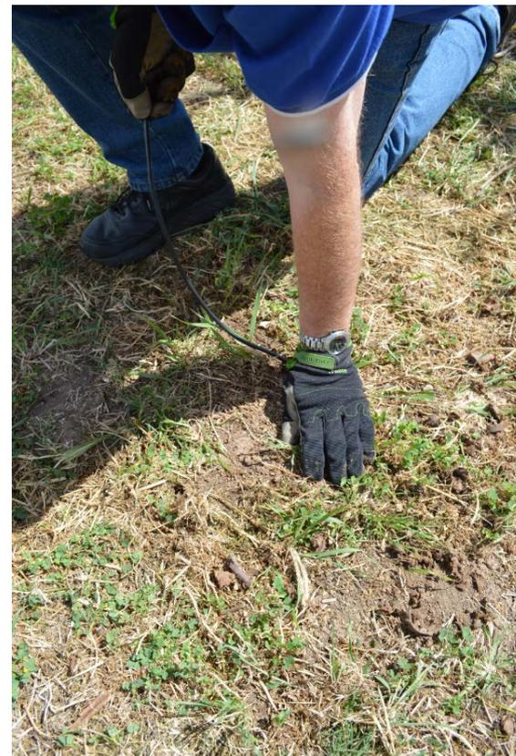
Insert the probe carefully into the hole pushing it all the way down until the top of the probe is level with the soil surface. The first sensor will now be located at 5cm depth.
