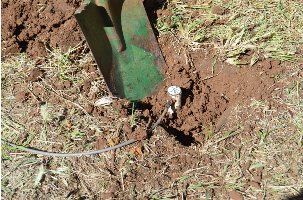
Excavate the soil adjacent to the probe to a depth of 20 cm. Wipe any soil or water from the probe using a piece of cloth. This will stop slippage of the Extraction Tool.
