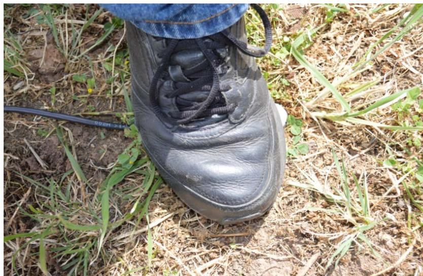
If the probe protrudes above the soil surface and you cannot push it any further by hand, gently step on it and use your body weight to push it into final position. Do not use unreasonable force.
