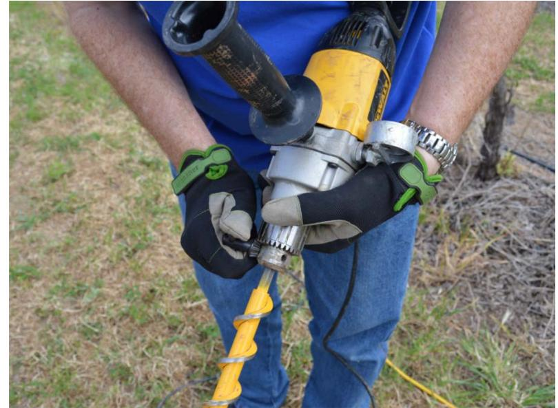
Insert the Tapered Auger into the drill and tighten the drill chuck.
