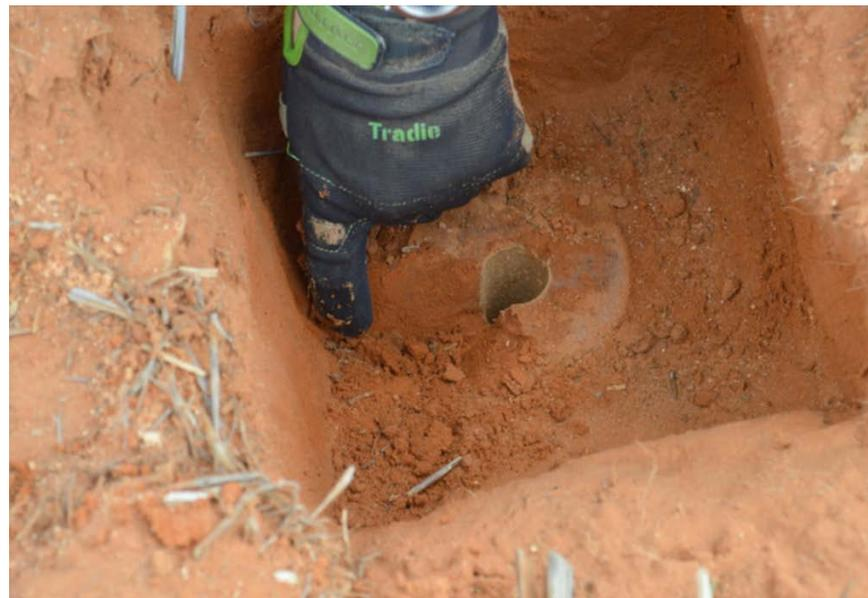
Place a finger carefully inside the augered hole to prevent soil entering and use a trowel to make a shallow 3cm deep trench to accommodate the probe cable.
