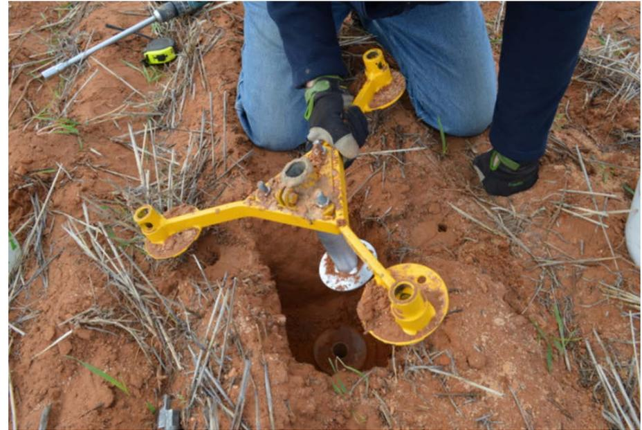
Before removing the tripod, remove any soil that may have landed in the hole around the Extension Tube. This will protect the augered probe hole during removal of the Tripod.
