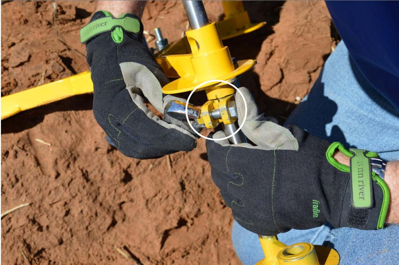
Re-tighten the nut and bolt (circled).
