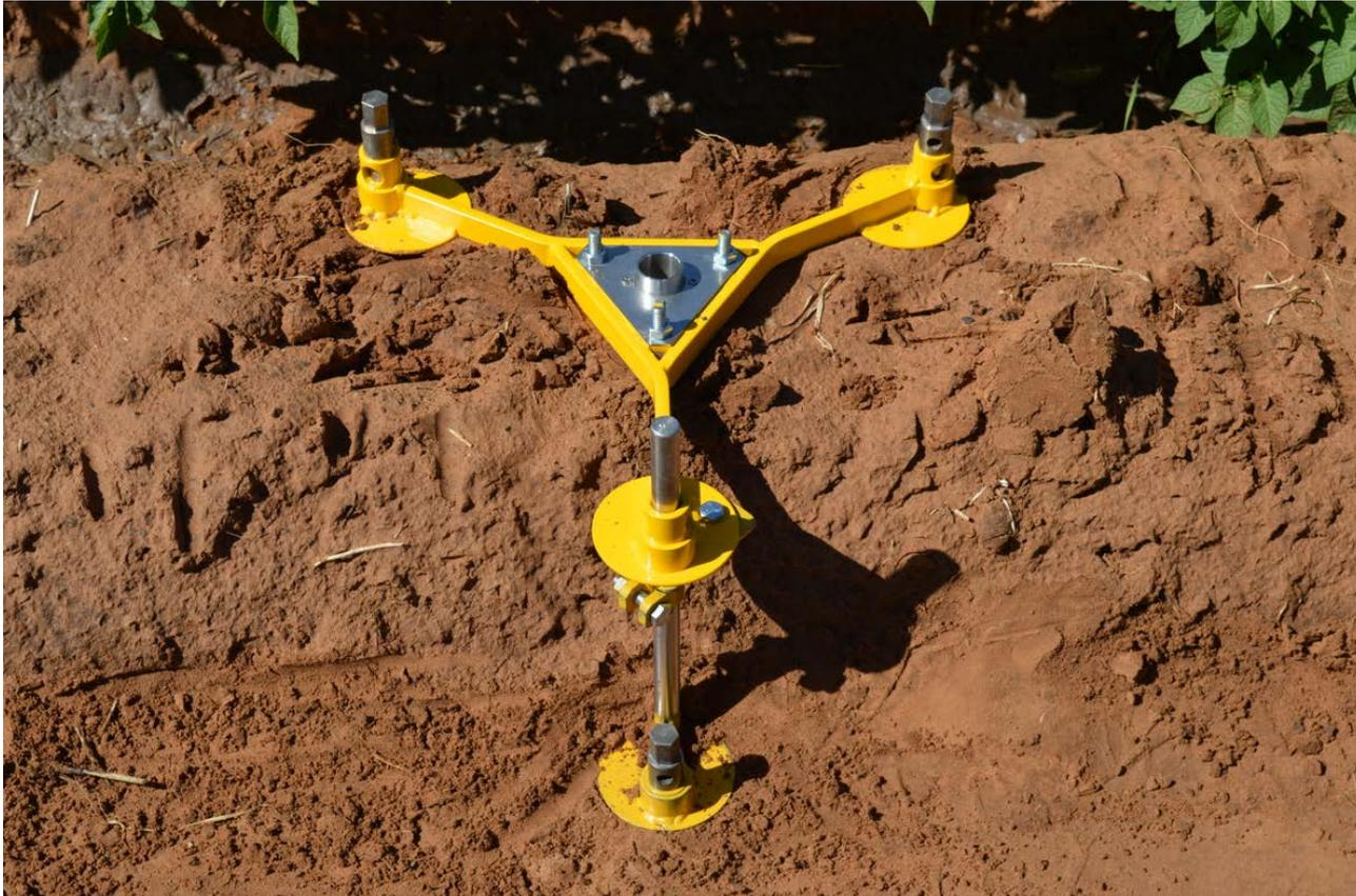
Two Tripod Feet are secured near the top of the hill, while the Extension Foot is secured at the bottom of the furrow.
